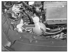
Fill the washer fluid in the tank if the washer fluid level is low.
