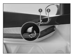
All the doors can also be locked from inside by pressing knob (1) on driver door and independently on other doors respectively.
