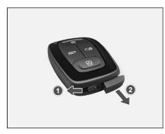
Slide the knob (1) to release the key. Pull the key blade (2) out.
