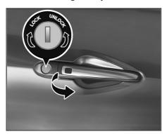
Insert the key in the slot and turn it clockwise to lock and anticlockwise to unlock the door.
