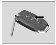
Press and hold approach light button for few sec until the tailgate is unlock.
