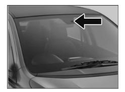
The integrated rain and light sensor is mounted on front windshield glass to sense rain and light.
