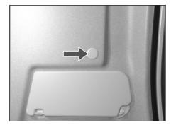
Mic is provided above the driver seat on roof.
