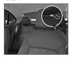
Adjust the head restraint so that it is as close to the head as possible and the center of the head restraint supports the back of the head at eye level. This will reduce the risk for injury to the head and neck in the event of an accident or similar situation.
