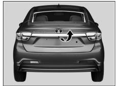
Press the tail gate opening button once (4) to unlock the tailgate with in authentication range (vehicle vicinity) of Smart key, then user has to press the tailgate switch within 30 sec.
