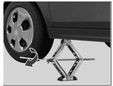
Lifting the rear wheel using jack
