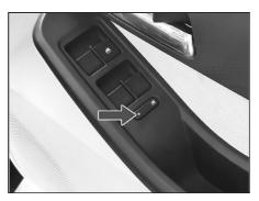
When switch is pressed, red light turns 'OFF'. The individual switches provided on other doors are not functional. It can be only operated by driver side switch.
