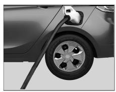
11. Charging Gun will be locked after switching on the DC charging station.
