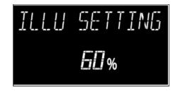
For Instrument Cluster illumination level settings, turn the Park Lamp 'ON' and then Press the 'SET' knob on instrument cluster.
