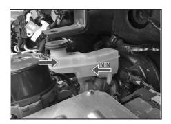
The level of the brake fluid should be between the 'MIN' and 'MAX' marks on the side of the brake fluid container. If the level falls below the 'MIN' mark, add recommended brake fluid.
