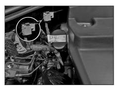
Isolation of high voltage components through low voltage Service Disconnect in case of emergencies.
