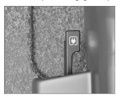
6. Open the protective cap on charging inlet.
