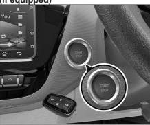
Start/Stop button is provided on the dashboard towards the left side of steering wheel.
