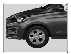
Put a piece of cloth between the spokes of the wheel cover and pull it outwards. Take out detached wheel cover from the wheel rim.
