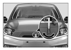
Lift the bonnet up. Pull the bonnet stay rod from its clip and engage the free end into the slot.
