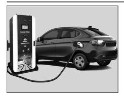
12. Normally the car starts charging automatically. If not, please refer Charging Gun's Fault Indication & Indication Priority Table on the charging station.
