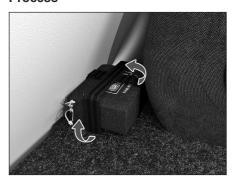
Remove the two Velcro as shown in figure and take out the puncture repair kit.
